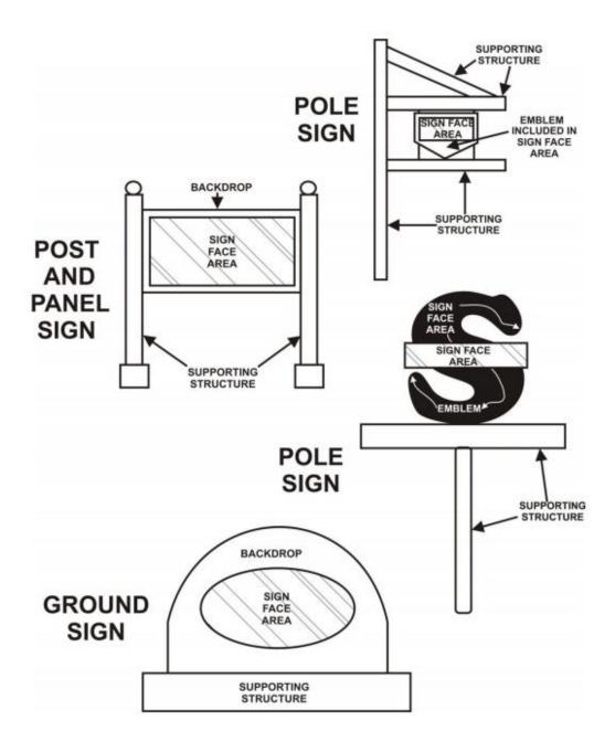
Figure Article 23 C. Sign Face Measurements
