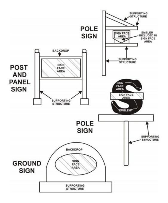
Figure Article 23 C. Sign Face Measurements
