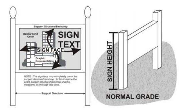
Figure Article 23 B. Diagrams of Sign Structure Components for Various Types of Sign Structures
