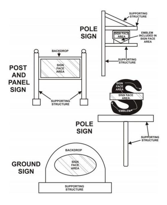
Figure Article 23 C. Sign Face Measurements
